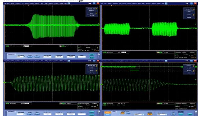
Figure 3: Beam signal of BPM after chopping. The upper plots: (left) the macro pulse of beam: 20  $\mu$ s/div; (right) the micro pulse of beam: 200 ns/div. The lower plots: (left) the rising edge of beam signal; (right) the falling edge of beam signal.
