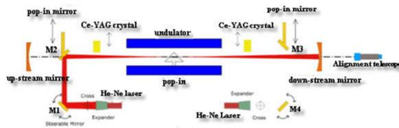
Figure 5: Layout of optical resonant cavity system.
