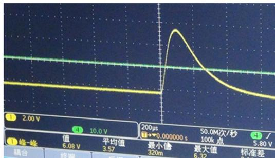
Figure 9: Output waveform from the Bolometer.
