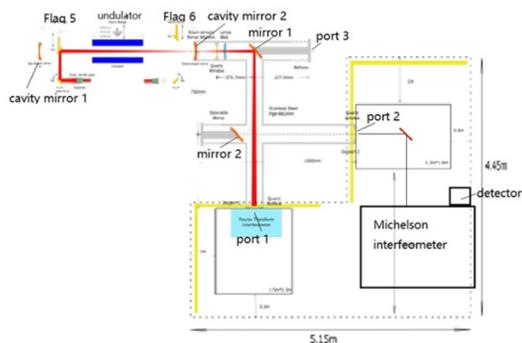
Figure 7: The layout of measuring system for testing the THz radiation.
