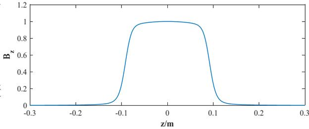
Figure 2: Solenoid field distribution.
