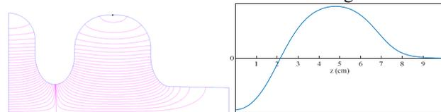
Figure 1: 1.4-cell cavity and field distribution.
