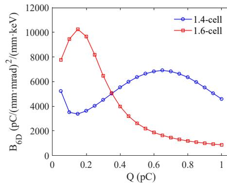
Figure 5: 6D brightness of electron beam generated by 1.4 and 1.6-cell RF guns.
