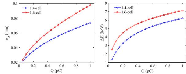
Figure 4: Bunch length (left) and energy spread (right) generated by 1.4 and 1.6-cell RF guns at  $70 \mu\text{m}$  and  $50 \text{ fs}$ .
