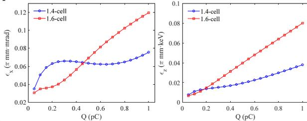
Figure 3: Transverse(left) and longitudinal(right) emittance by 1.4 and 1.6-cell RF guns at  $70 \mu\text{m}$  and  $50 \text{ fs}$ .
