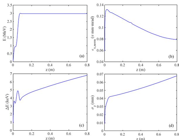
Figure 6: Beam parameters as a function of  $z$ . (a) Beam energy; (b) Normalized transverse emittance; (c) RMS energy spread; (d) Bunch length.
