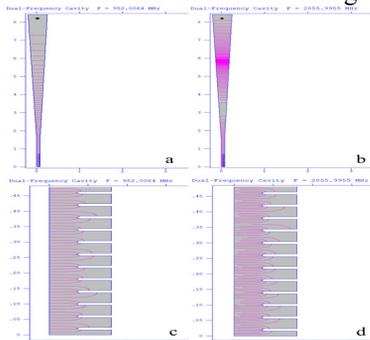
Figure 5: a, b are the electric fields of TM010, TM020 mode respectively in cavity. c, d are the Electric fields of TM010, TM020 mode respectively at the grid.
