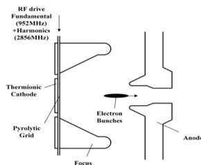
Figure 3: Diagram of RF-gated gridded Egun.
