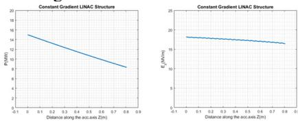
Figure 10: RF power and field strength along the accelerating section.
