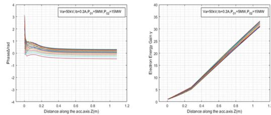
Figure 11: Beam phase trajectory and energy gain.
