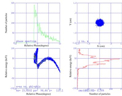
Figure 12: Current profile, transverse beam size, longitudinal phase space and Energy spectrum at exit of the LINAC.
