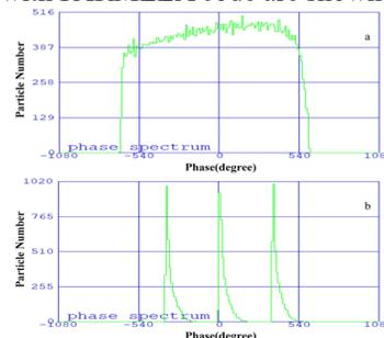
Figure 7: (Up) current profile at exit of the DC gun. (Down) current profile at exit of the RF-gated gridded gun.
