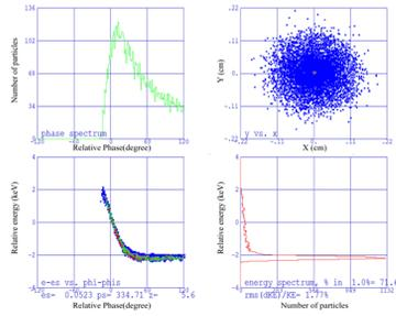
Figure 8: Current profile, transverse beam size, longitudinal phase space and Energy spectrum for RF-gated gridded gun.
