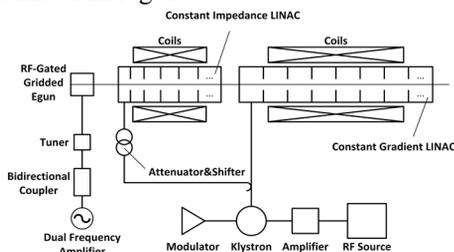
Figure 1: Schematic diagram of the THz FEL injector based on a RF-gated gridded electron gun.
