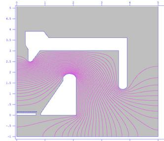
Figure 6: Model of RF-gated gridded gun.
