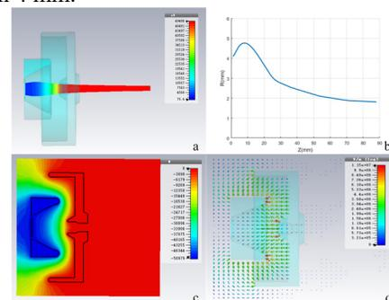
Figure 2: a. 3D model of the DC gun with trajectory. b. Envelope of the beam. c. Potential distribution. d. Electric field distribution.
