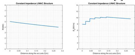
Figure 9: RF power and field strength along the bunching section.
