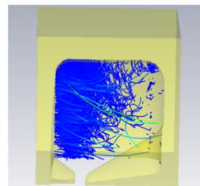
Figure 6: Multipacting occurs when the cathode gradient is 16 MV/m. Most of the particles locate at the upper corner of the anode plate.
