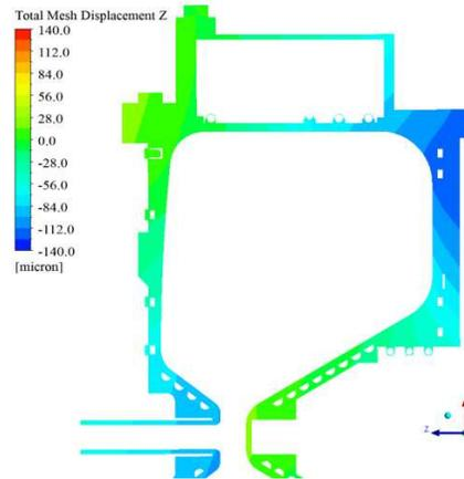
Figure 4: Contour plot of the deformation of the gun profile.
