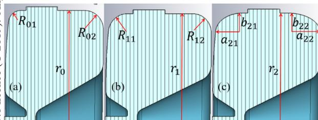
Figure 8: (a) The present gun shape. (b) new gun shape 1. (c) new gun shape 2.
