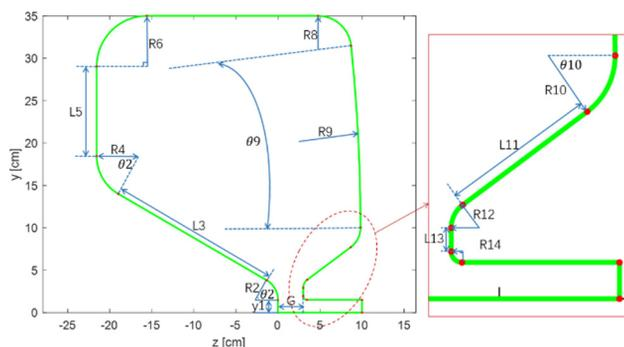
Figure 1: Cavity profile parameterized in CST.
