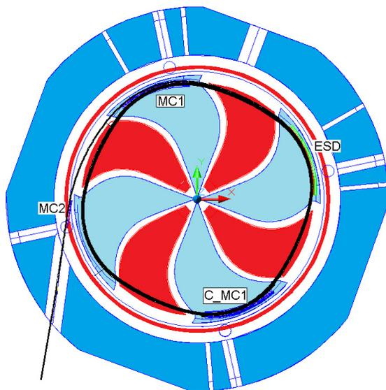
Figure 9: Extraction system of SC230: ESD –electrostatic deflector, MC1 – first magnetic channel, MC2 – second magnetic channel, C\_MC1 – compensator of the first harmonic induced by the magnetic channels.
