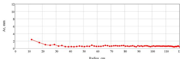
Figure 8: Amplitudes of radial betatron oscillations of the reference particle.
