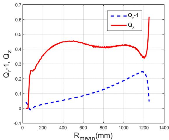
Figure 2: Vertical and radial betatron tunes in SC230.
