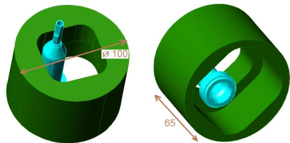
Figure 6: Location of the ion source in the central plug.
