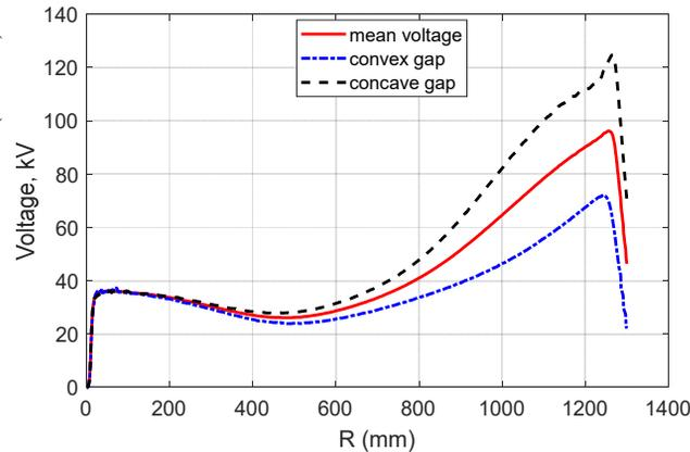
Figure 4: Accelerating voltage along radius.
