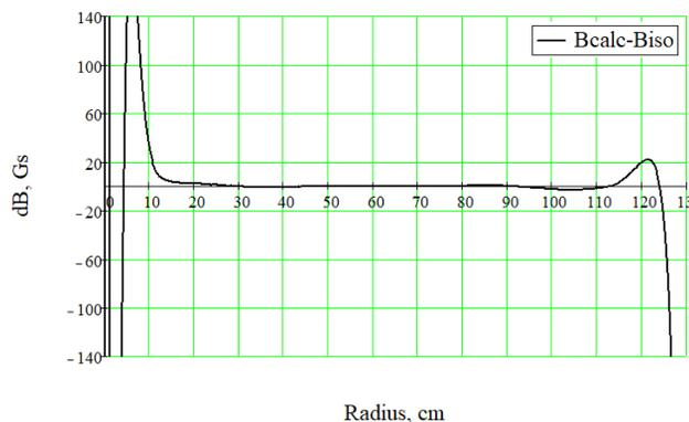
Figure 1: Difference between average magnetic field and isochronous curve.
