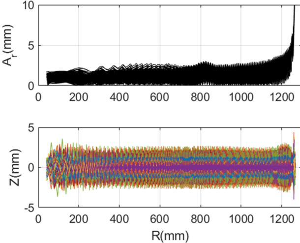
Figure 3: Amplitudes of radial oscillations and vertical motion of the beam.
