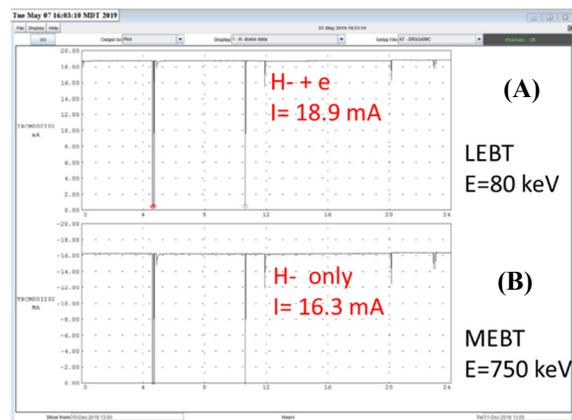
Figure 2: 24 hours charts of stable beam currents recorded at H<sup>-</sup> beam injector: LEBT (A) and MEBT (B).
