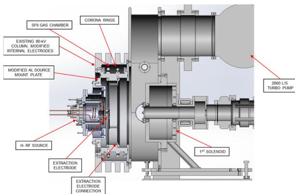
Figure 4: Cross section of SNS RF ion source with 80 kV extraction electrostatic column and two solenoid LEBT is shown.
