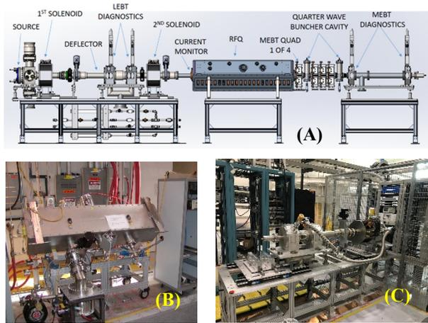
Figure 3: (A) Side view of new RFQ test stand model is shown. (B) new RFQ in preparation for high power test and commissioning and (C) recently assembled LEBT with the 35 kV high voltage platform.
