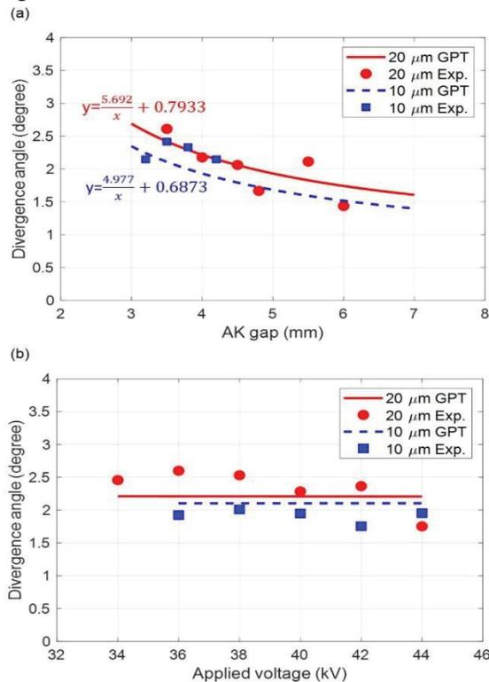
Figure 2: Measured and simulated divergence angles at different AK gaps and applied voltages. (a) The AK gap was varied from 3 to 6 mm, and the applied voltage was fixed at 40 kV. (b) For the 20 and 10 μm pyramids, the AK gap was fixed at 4 mm and 3.6 mm, respectively, while the applied voltage was varied.
