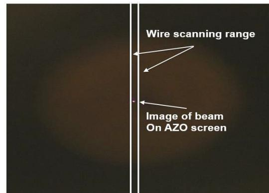
Figure 4: Snapshot of the beam at a distance of 16 mm from the magnetic center of the lens. The white bars indicate the wire scanning range.
