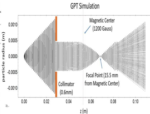
Figure 5: GPT simulation of the beam converging to a 3  $\mu\text{m}$  spot size at a distance of 15.8 mm from the magnetic center.
