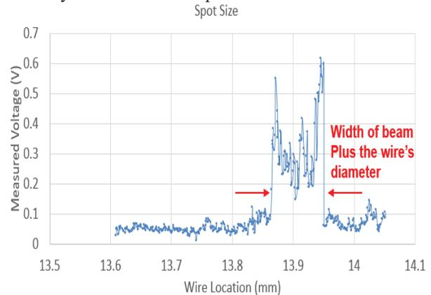
Figure 6: Graph of the measured voltage on the copper wire versus the location of the wire. Showing a spot size of 5.72  $\mu\text{m}$ .
