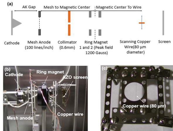
Figure 3: (a) Schematic of the focusing studies. (b) Photograph of the focusing study setup. (c) Photograph of the copper wire holder. The wire is 80 μm in diameter.
