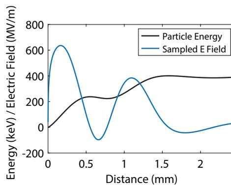
Figure 5: Sampled on-axis electric field (blue) and the resulting change in electron energy (black) for 1 MW of input gyrotron power and a launch phase of 60 degrees.
