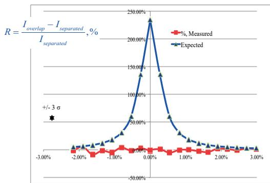
Figure 2: Predicted and measured relative increase in the radiation of electron beam by overlapping ion beam as a function of relative error in relativistic factors.
