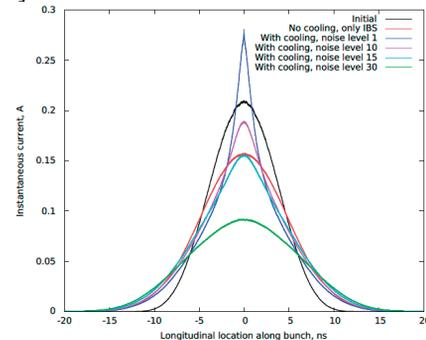
Figure 5: Evolution of the 26.5 GeV/u ion bunch profile in RHIC. Black - initial profiles at  $t=0$ . All other profiles are shown at  $t=40$  minutes. Red – evolution of witness bunch without cooling; blue – cooled with e-beam having natural shot noise; crimson - cooled, e-beam with 10 time increase in amplitude of shot noise; cyan - cooled, e-beam with 15 time increase in amplitude of shot noise; and green - , e-beam with 30 time increase in amplitude of shot noise.
