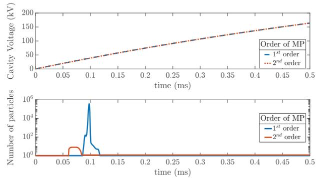
Figure 5: Cavity voltage and the number of secondary electrons as a function of time: 1<sup>st</sup> and 2<sup>nd</sup> order MP with the maximum coupling, available power of 4 kW, and adjusted SEY for Nb.
