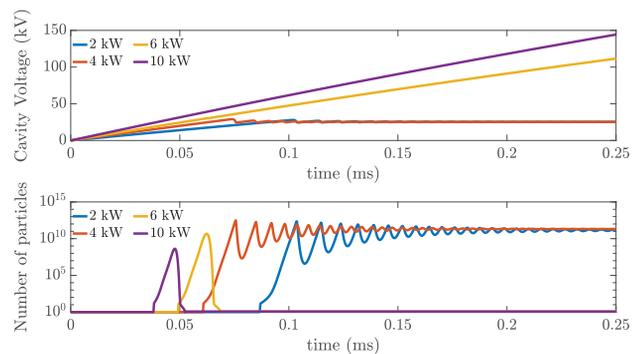
Figure 6: Cavity voltage and the number of secondary electrons as a function of time with the presence of the 2<sup>nd</sup> order MP: fully inserted FPC, SEY for Nb and various values of the input power.
