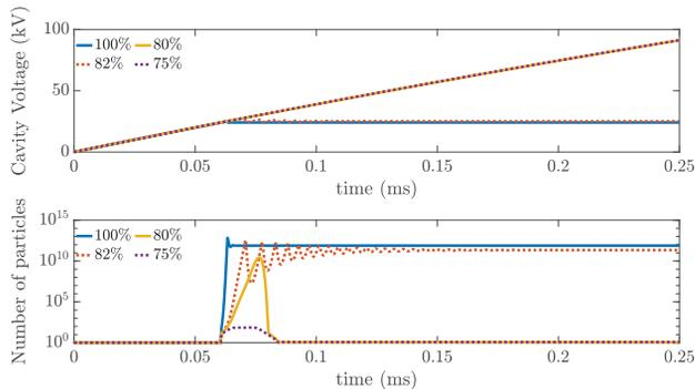
Figure 7: Cavity voltage and the number of secondary electrons as a function of time with the presence of the 2<sup>nd</sup> order MP: fully inserted FPC, 4 kW input power and different uniform scaling of the SEY for Nb.
