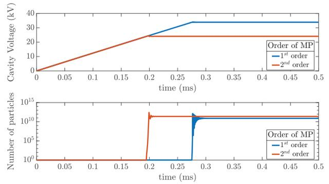
Figure 4: Cavity voltage and the number of secondary electrons as a function of time: 1<sup>st</sup> and 2<sup>nd</sup> order MP with the FPC being inserted half-way in, maximal available power of 4 kW, and SEY for Nb.
