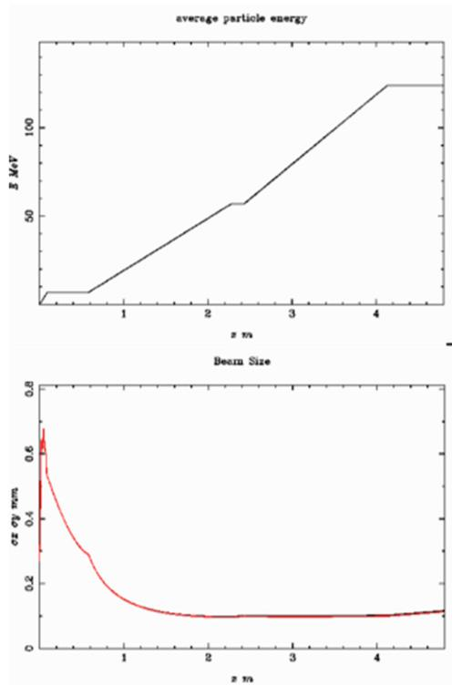
Figure 3: Energy boosting (up) and beam size (down) for 250pC along the photoinjector injector.
