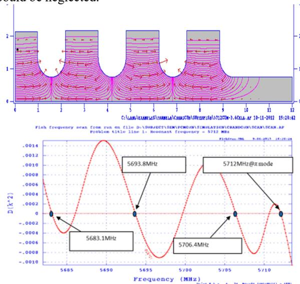
Figure 1: field distribution of  $\pi$  mode (upper) and frequency for four different modes (lower).
