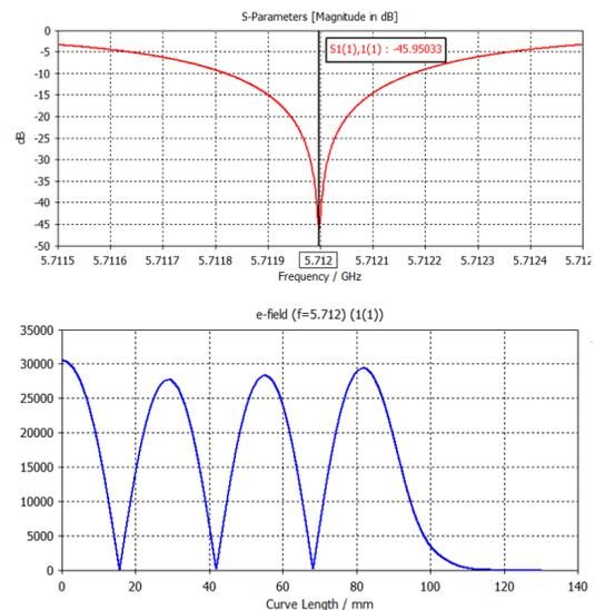
Figure 6: Frequency, coupling coefficient and field flatness.
