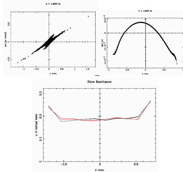
Figure 4: Simulation results of 250pC bunch charge. Transverse phase space (upper left), longitudinal phase space (upper right), slice emittance dist. (lower).
