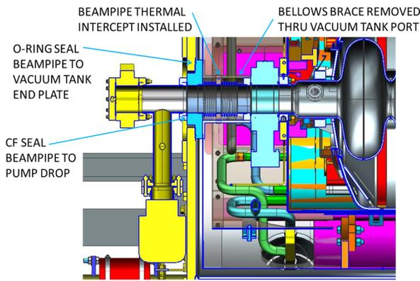
Figure 1: Some of the recent design features in the new PPU cryomodules [3].
