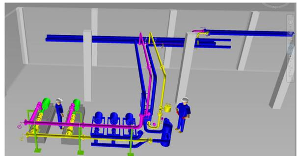
Figure 2: Ring Service Building power supply water cooling system upgrade. Existing pumps are shown in blue. They will be replaced by the pumps shown in green.
