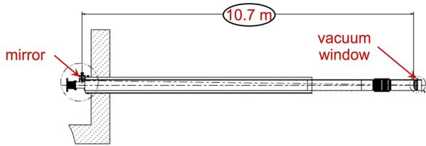
Figure 3: Cross section of the last part of the Ring Injection Dump beam line, showing the main components of the imaging system.
