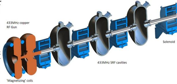
Figure 2: Conceptual design of the RF Gun based injector.
