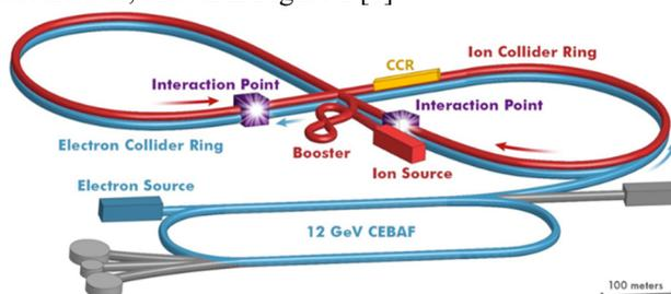
Figure 1: A schematic of the JLEIC accelerator complex.
