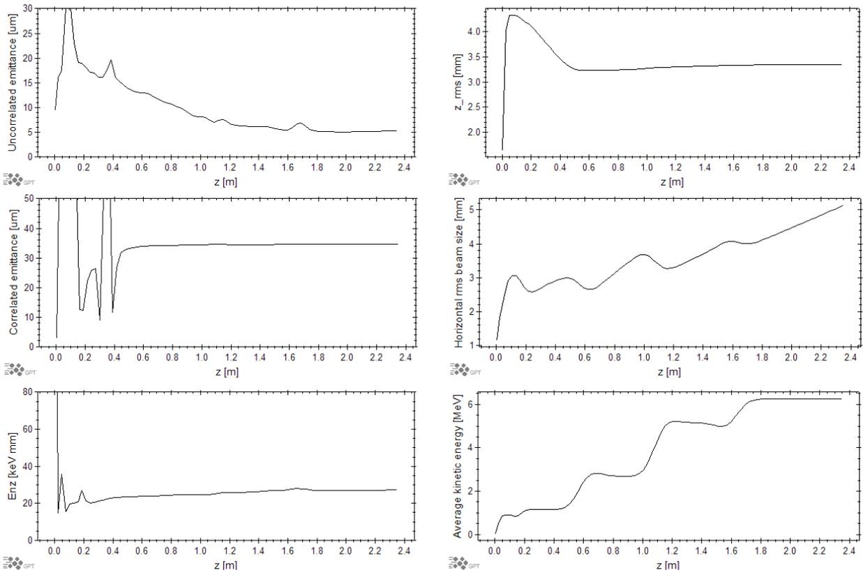
Figure 4: Beam evolution along the injector beamline.
