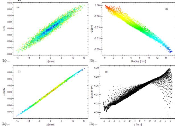
Figure 5: Phase Space at the injector exit, color-coded on angular momentum as shown in (b). (a) Horizontal phase space, (b) radial phase space, (c) Horizontal uncorrelated phase space, (d) longitudinal phase space.
