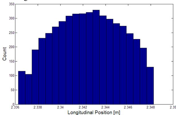
Figure 6: Longitudinal bunch profile at the injector exit.
