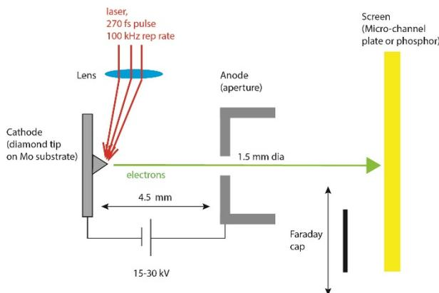
Figure 2: The schematic of the strong-field photoemission test stand.
