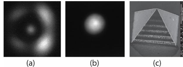
Figure 4: The emission pattern observed on the MCP screen for (a) lower laser intensities; (b) higher laser intensities. (c) The SEM image of a pyramid damaged by the laser light.
