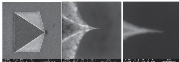
Figure 1: Scanning electron microscope (SEM) images of a diamond nano-tip at different magnifications.
