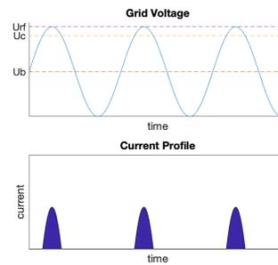
Figure 2: Illustration relating grid voltages to current profile of bunches.
