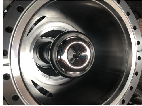
Figure 3: Thermionic electron source design, and assembly at Xelera’s facility.
