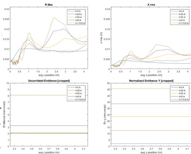
Figure 6: Simulations of transverse size and emittance for 130 pC bunch charges at various magnetizations.
