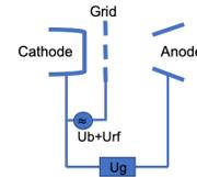
Figure 1: Conceptual cathode, grid, anode diagram.  $U_g$ : gun voltage.
