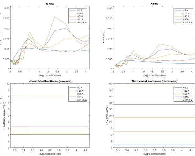
Figure 5: Simulations of transverse size and emittance for 1 pC bunch charges at various magnetizations.
