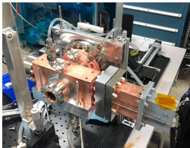
Figure 1: Picture of RadiaBeam's thermionic gun.
