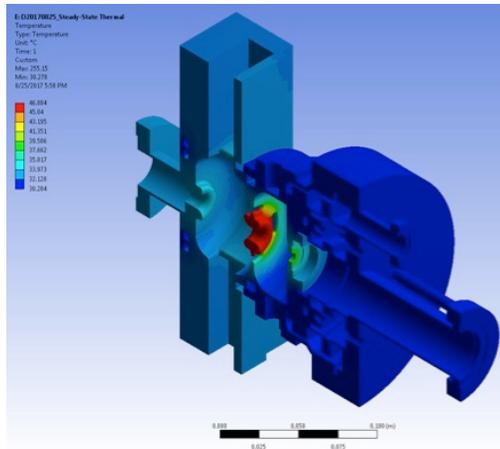
Figure 4: ANSYS thermal simulation of the gun.
