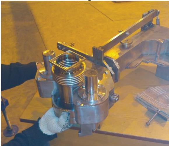
Figure 5: End of accelerator vacuum flange with added bellows.
