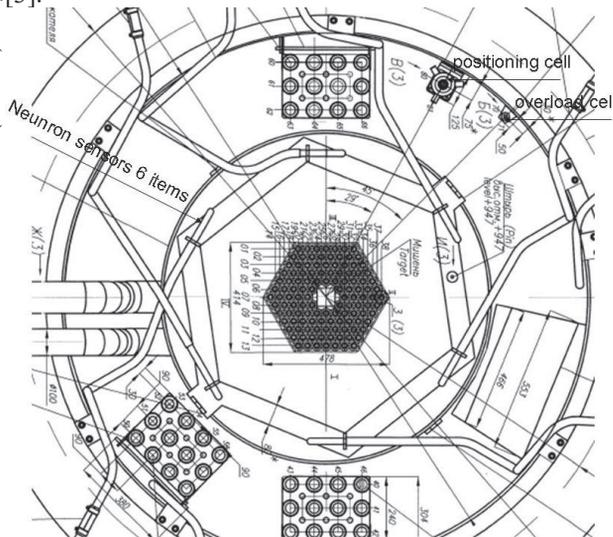
Figure 1: Layout of the SCA Neutron Source neutron flux measurement system.
