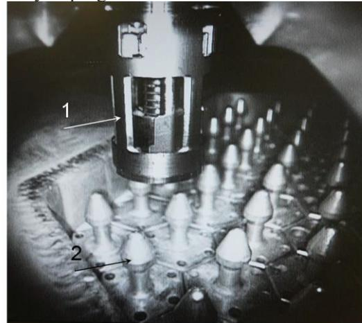
Figure 7: Screen of a fuel reloading machine operator. 1 – a manipulator grip; 2 – a beryllium core element
