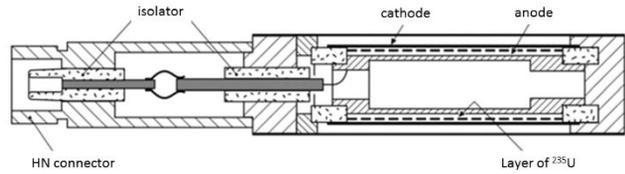
Figure 2: NSC KIPT SCA Neutron Source neutron detector scheme.
