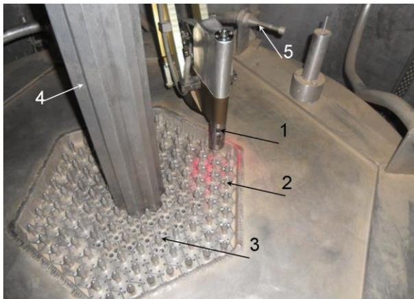
Figure 6: Service of an active zone. 1 – a manipulator grip; 2 – a beryllium core element; 3 – a core fuel cell; 4 – a target; 5 – a neutron sensor
