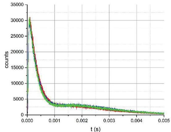
Figure 4: The pulse response of CFUF34 detectors.
