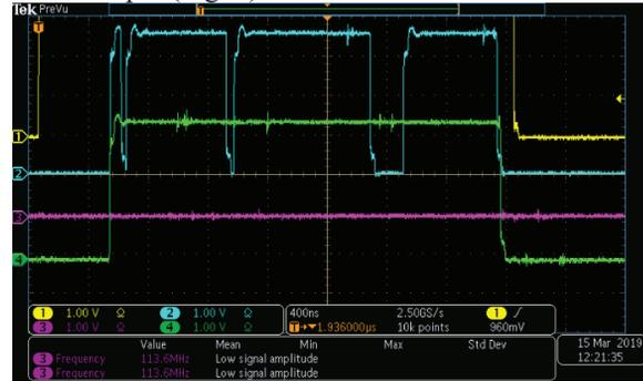
Figure 3: CFUF34 detectors signals. The yellow curve is synchronizing pulse, green & blue are for unshielded detectors, and magenta is a lead shielded detector.
