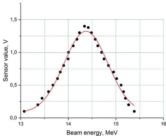
Figure 4: Electron beam energy distribution after injection section.
