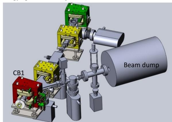
Figure 3: Layout of the chicane and beam dump.
