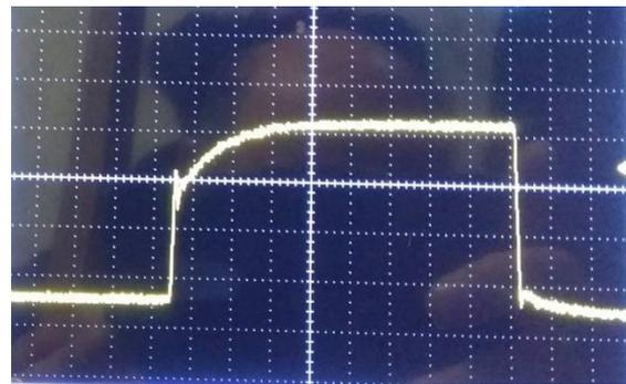
Figure 2: The gun current pulse shape.
