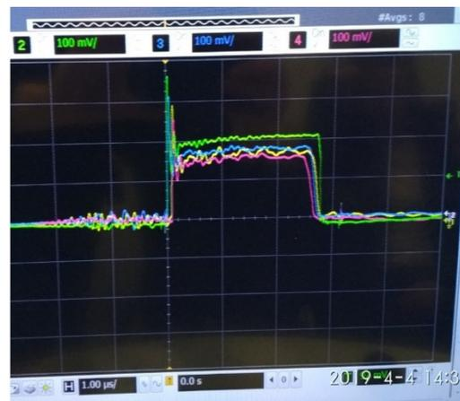
Figure 6: Beam current monitor signals: green – FCT2 (chicane entering), blue - FCT3 (after chicane), yellow – FCT4 (ending of linac regular part), red – FCT5 (after first bending to neutron target).
