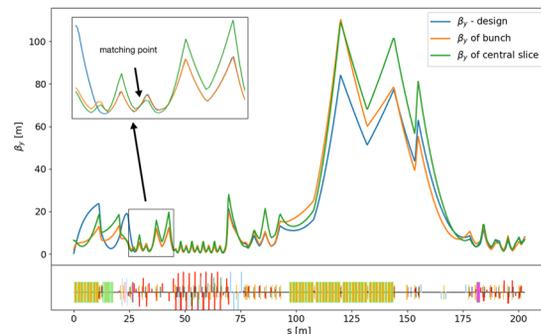
Figure 1:  $\beta_y$  of the first 200 m of the EuXFEL accelerator: design  $\beta_y$  (blue line),  $\beta_y$  of whole bunch from tracking with SC. (orange line),  $\beta_y$  of the central slice (green).
