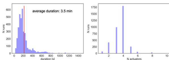
Figure 3: Distribution of optimizations duration (left) and number of actuators used in individual optimizations (right) for 16 months of usage.
