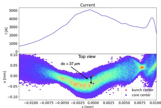
Figure 7: The electron beam parameter in from of SASE2 undulator, the beam energy 14 GeV, 250 pC [16].
