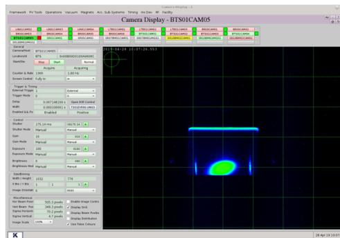
Figure 2: Image of YAG screen illuminated by beam.
