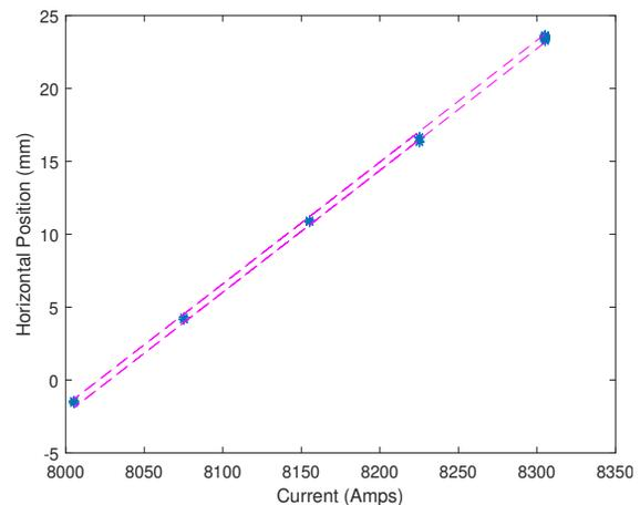
Figure 8: Current of final septa steering magnet vs beamspot position.
