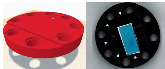
Figure 3: Film holder CAD model designed in Tinkercad for 3D printing (Left) vs the real thing with film (right).
