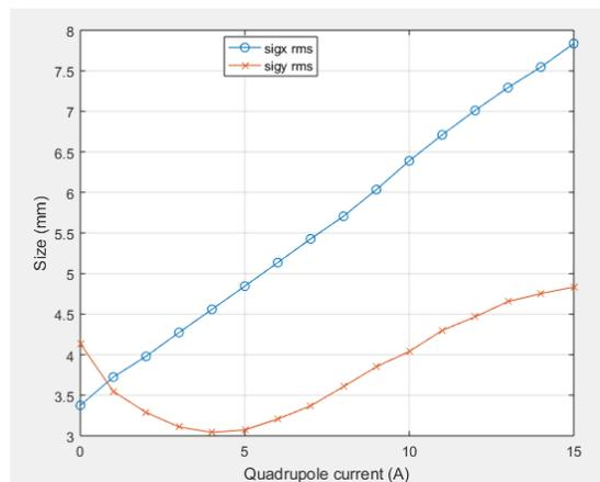
Figure 6: Influence of the quadrupole current on the beam size.
