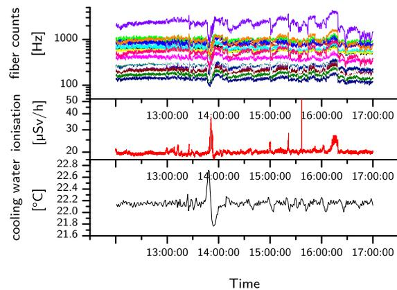
Figure 7: Count rates of the 18 fibers mounted on RTM1 compared to the ionisation chamber at 14 MeV and the cooling water temperature.
