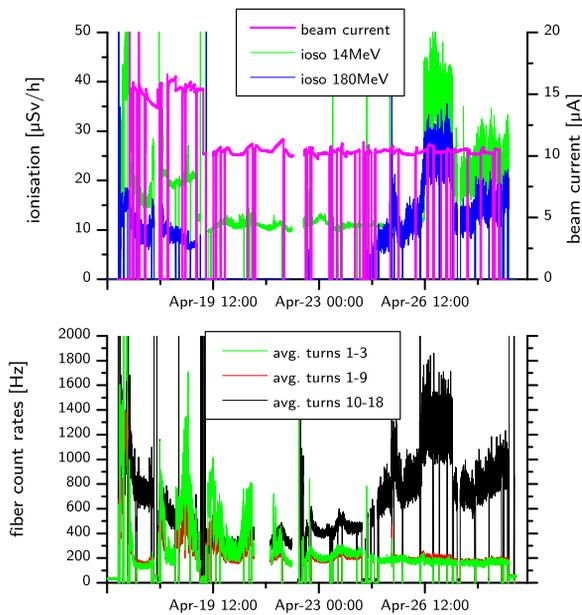
Figure 5: Beam losses at RTM1. Top: beam current and ionisation chambers in Hall A of MAMI. Bottom: Average count rates of turns 1–3, turns 1–9 and turns 10–18 of the fibers developing in different directions.
