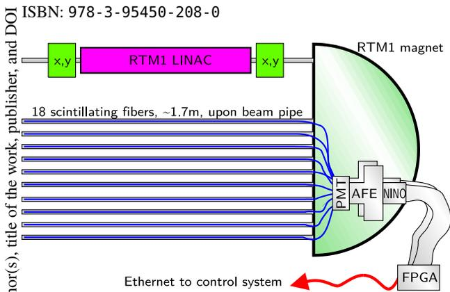
Figure 2: Schematic drawing of the detector system [5] (PMT: photo multiplier, AFE: analogue front end).
