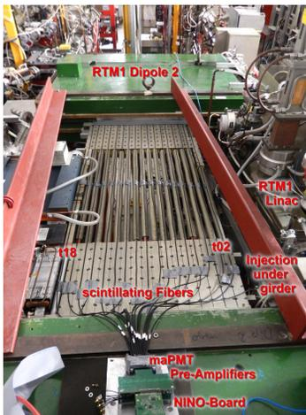
Figure 3: Photo of the fibers attached to the return paths of RTM1 [5]. Linac on the right side, turn 1 (injection) under the red girder, then turn 2–18 from right to left.
