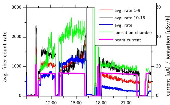
Figure 6: Comparison of the beam losses detected with the ionisation chamber (green) and the average count rates of the fibers for turns 1–9 (red) and turns 10–18 (black) on the first day.
