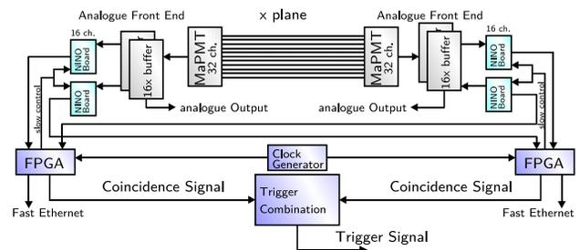
Figure 4: Block diagram of the data acquisition system. The FPGA board (MYiR Z-turn with Xilinx Zynq-7220, 100 MHz) is used to perform the coincidences, to count the individual and coincidence rates, to generate regions of interest, and to adjust the thresholds and pulse widths of the NINO Chip. Events can be accumulated with timestamps in an event builder. Read out is done via fast Ethernet. Only half of the electronics were used for the measurements.
