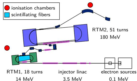
Figure 1: Position of the two ionisation chambers with respect to the beam line and the accelerator components in Hall A of MAMI and the area with the fibers at the RTM1.
