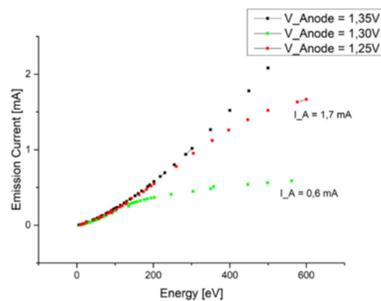
Figure 5: Measured electron beam current as a function of different cathode heat power and beam energy.
