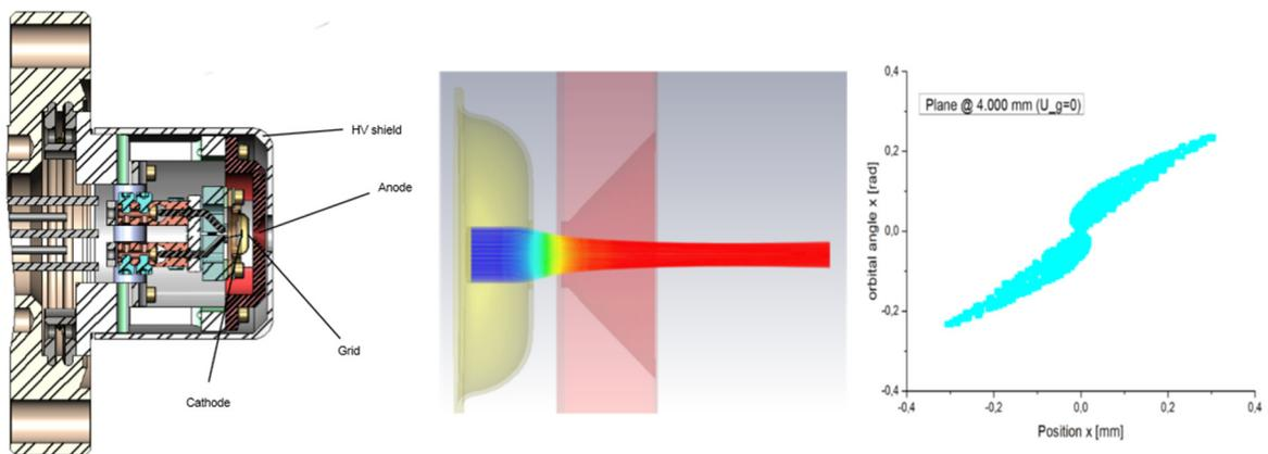
Figure 6: Technical layout of the electron source (left) and simulated electron extraction, beamlet formation (middle) and phase space distribution of electron beamlet 4.0 mm behind extraction grid (right).
