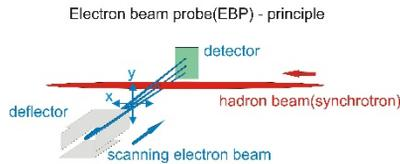
Figure 1: Layout of the electron beam probe (EBP).
