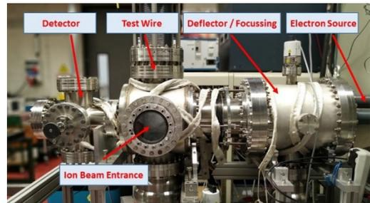
Figure 7: Image of the EBP test bench at Goethe-University after assembling, before applying the bake-out procedure.
