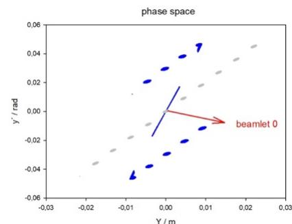
Figure 4: Detector signal in phase space ( $Y - Y'$ ) at 0.5 m from the electron source ( $E_e = 5\text{ keV}$ ). Grey – simulation without, blue – simulation with proton beam potential.
