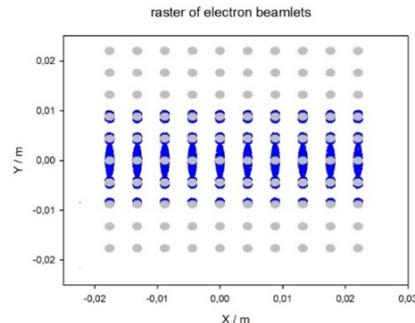
Figure 3: Detector signal ( $X - Y$ ) at 0.5 m from the electron source ( $E_e = 5\text{ keV}$ ). Grey – simulation without, blue – simulation with proton beam potential.
