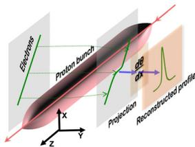
Figure 2: Transverse beam profile measurement with a tilted sheet of coulomb scattered electrons (W. Bloklund).
