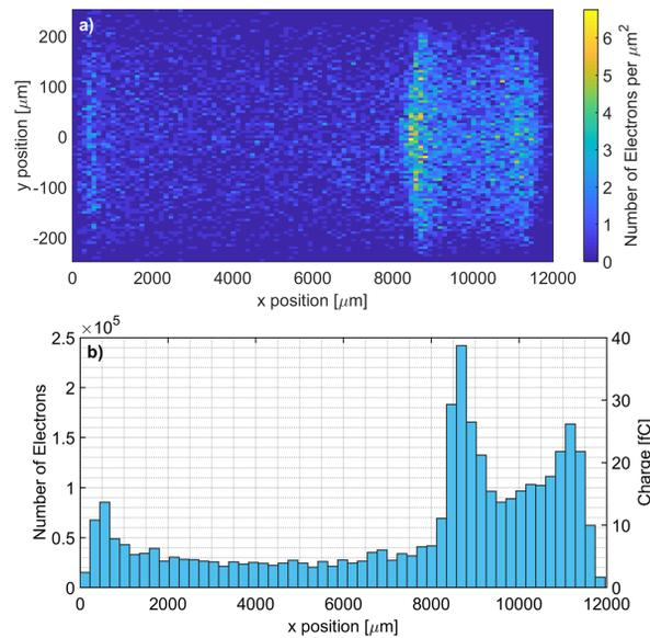
Figure 1: a) Electron beam distribution in  $x$  and  $y$  dimensions. The number of electrons per  $\mu\text{m}^2$  is displayed with a bin size of  $(120 \times 5) \mu\text{m}^2$ . b) Electron beam distribution in  $x$  dimension integrated over the whole  $y$  range. A bin width of  $225 \mu\text{m}$  was chosen to match the detector readout channel width. Both distributions are displayed at the position of the detector for a 0.5 pC ACHIP working point.
