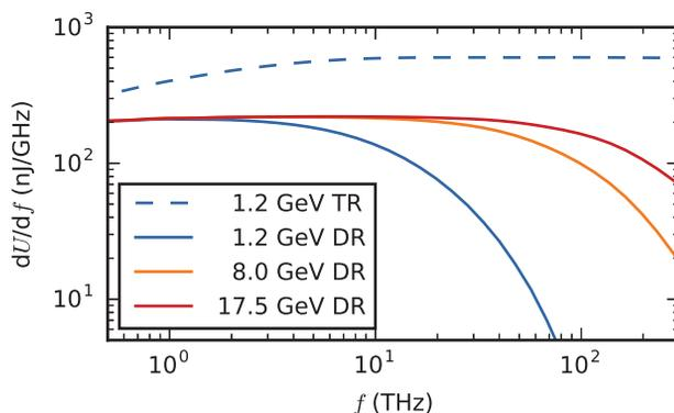
Figure 1: Numerically calculated single electron spectral intensity of transition and diffraction radiation according to Eq. (25) in Ref. [4]. A circular screen with 16 mm radius and 5 mm aperture for DR was used.
