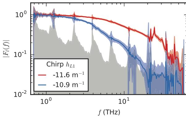
Figure 5: Measured form factor moduli  $|F_l|$  and their standard deviations for two different compression settings for the electron energy chirp  $h_{L1}$ . The gray area indicates the sensitivity limit.
