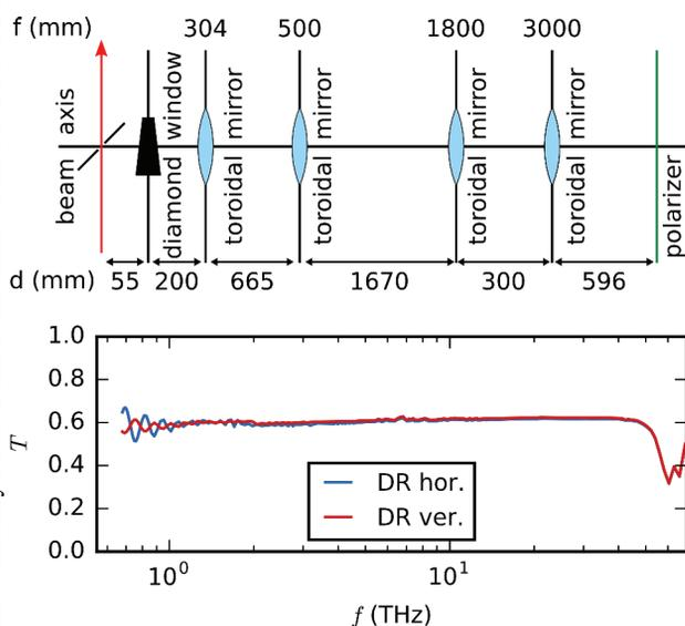
Figure 3: Optical setup (top, not to scale) and transmission as function of frequency (bottom) of the THz beamline. See text for details.
