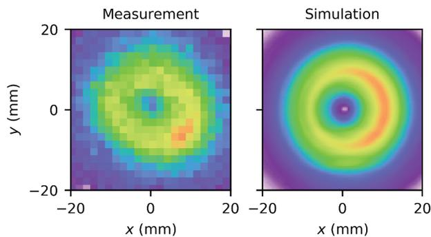
Figure 4: Measurement and simulation of the 2D beam profile at the end of the THz beamline.
