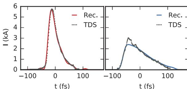
Figure 6: Current profiles measured with the TDS together with the current profile reconstruction from the form factors shown in Fig. 5.
