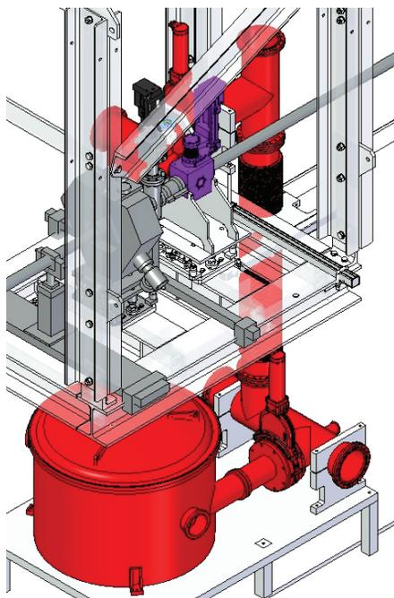
Figure 2: Sketch of the THz beamline at European XFEL. The electrons pass the station from the right to the left through the beam pipe shown in gray. Purple marks the screen station with the mover while the THz beamline and spectrometer are displayed in red.
