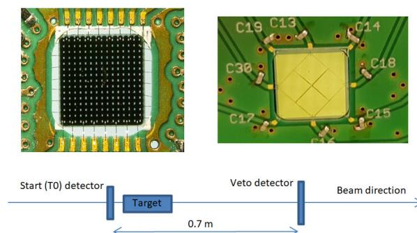
Figure 1: Arrangement of the scCVD diamond sensors in the HADES experiment. In the upper left a close-up picture of the T0 sensor is shown. The metallization which is arranged in sixteen stripes is clearly visible. The upper right corner shows a close-up picture of the scCVD diamond based veto detector with a boxed shaped metallization.
