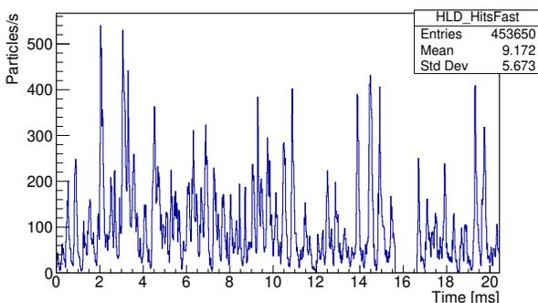
Figure 5: Micro-spill time structure of the particle rates.
