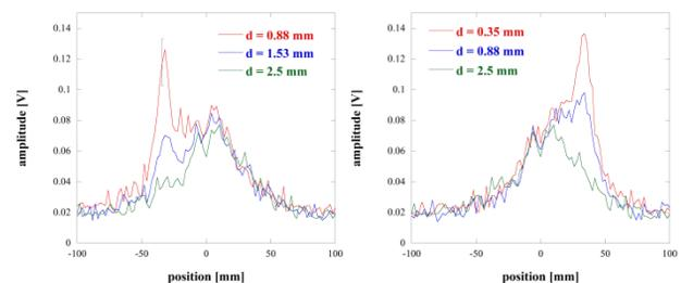
Figure 3: Beam position dependence of the radiation intensity. The beam was steered to -1.05, -1.65 mm (left) and +1.35, +1.85 mm (right). An error bar represents the typical standard deviation of the measured signal.
