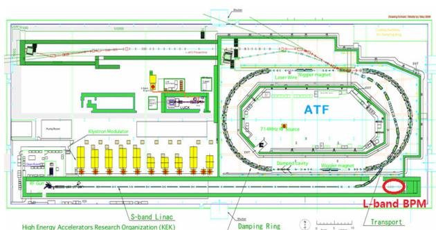
Figure 1: The layout of ATF. The red circle shows the installation location of three L-band BPM.
