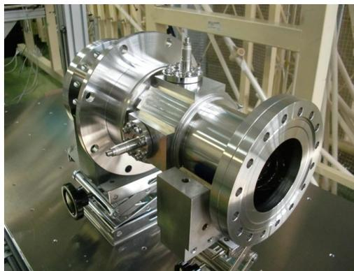
Figure 2: The fabricated L-band BPM.
