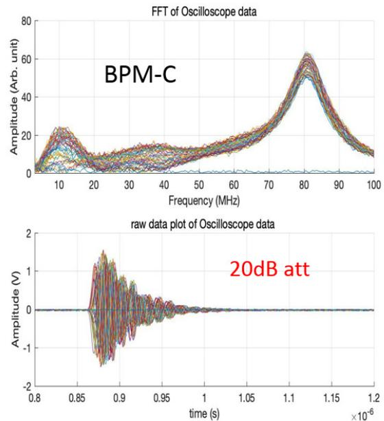
Figure 6: FFT of IF signal for L-band BPM-C.
