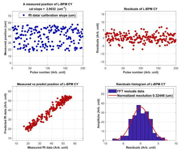
Figure 8: The measured position resolution of BPM-C y-port is 324nm with 1.6nC beam charge condition.
