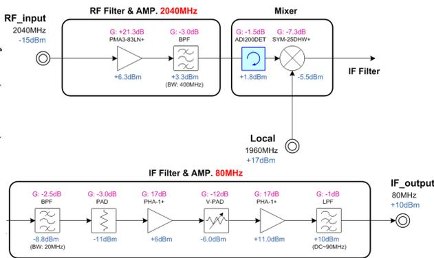
Figure 4: The first stage electronics scheme for L-band BPM signal processing.
