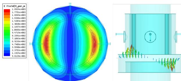
Figure 3: The HFSS RF simulation results of L-band BPM.
