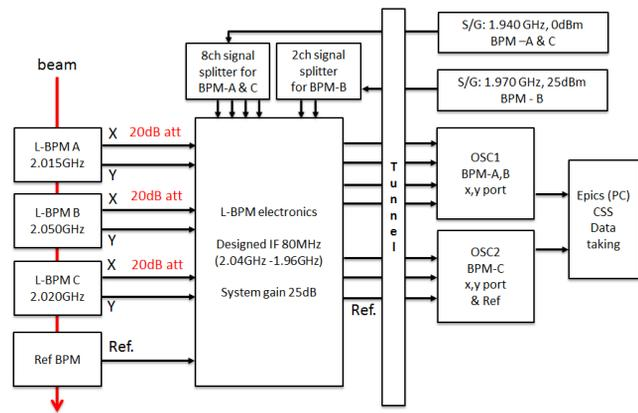
Figure 5: The beam test scheme of L-band BPM entire system.
