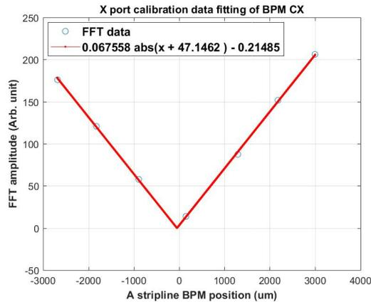
Figure 7: L-band BPM-C x-port calibration factor. The calibration run performed under 20dB attenuation case.
