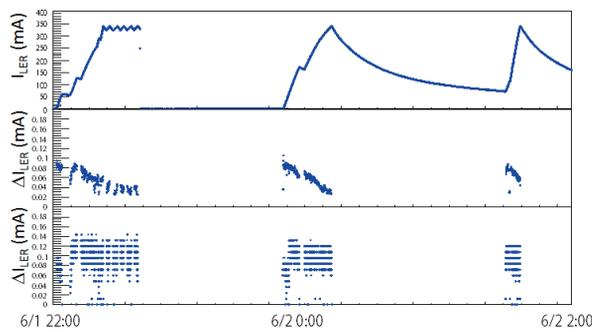
Figure 2: Time chart of operation current and injected currents at LER: The top plot shows the operation current. The middle and bottom plots are the injected currents determined with ordinary and new methods, respectively. The data from June 1st 22:00 to June 2nd 2:00 in 2018 are shown.
