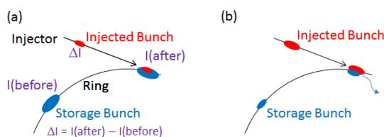
Figure 5: Illustrations of the relation between the injected bunch and storage bunch (a) and their beam-beam kick (b): the injected current,  $\Delta I$ , is determined as the bunch current after injection,  $I(\text{after})$ , minus that before injection,  $I(\text{before})$ . The injection archiver system records  $I(\text{before})$ ,  $I(\text{after})$ , and  $\Delta I$ .
