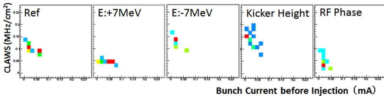
Figure 4: Two-dimensional plots for bunch current of Injection-bucket before injection and beam background rate at IP: the data in the injection conditions of normal parameters, injection bunch energy +7 MeV and -7 MeV, injection kicker height -0.75 mm, and RF phase at HER +4 degrees are shown. The number of entries in each bin is illustrated with colors. The red indicates large entries while the blue indicates a few entries.
