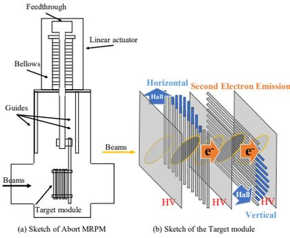
Figure 2: Sketch of Abort MRPM (a) and its target (b).
