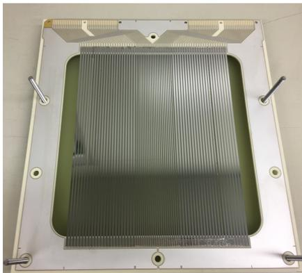
Figure 4: Horizontal target base after YAG laser cut.
