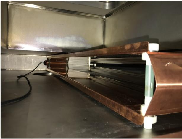
Figure 1: Photo of full-aperture bunch monitor. 100 mm(W)×75 mm(H)×158 mm(L).
