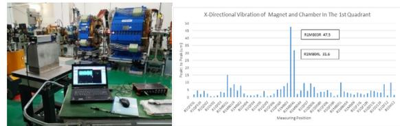
Figure 7: Laser vibration measurement system.
