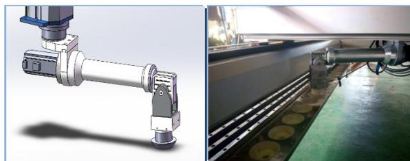
Figure 2: Remote target drop-and-grab device.
