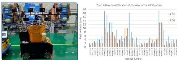
Figure 6: Visual vibration measurement.
