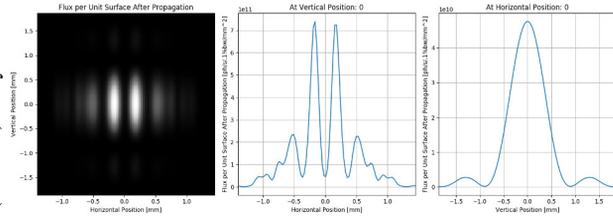
Figure 2: Image and intensity distribution obtained from 3-slit imaging system.
