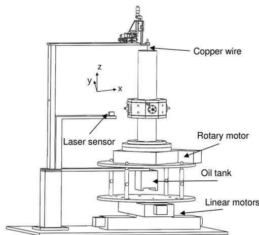
Figure 2: Picture of the test bench.
