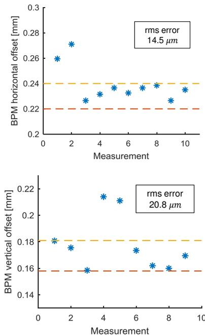
Figure 4: Measured electric offsets of the button BPM.
