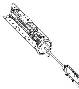
Figure 3: Mechanical schematic of CSNS wire scanner.
