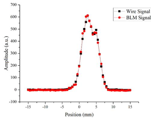
Figure 9: Beam profile plotted by wire signal and downstream BLM signal.
