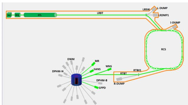
Figure 1: Schematics of the CSNS complex.
