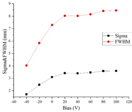
Figure 7: Calculating beam size varying with the bias.
