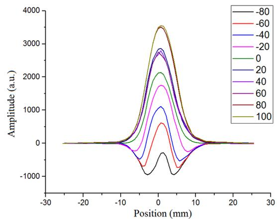
Figure 5: Horizontal profile measurement results under different bias voltage at CSNS-MEBT.
