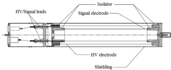
Figure 4: Schematic of the BLM at CSNS.
