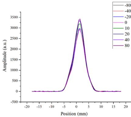
Figure 8: Horizontal profile measurement results under different bias voltage at CSNS-LRBT.
