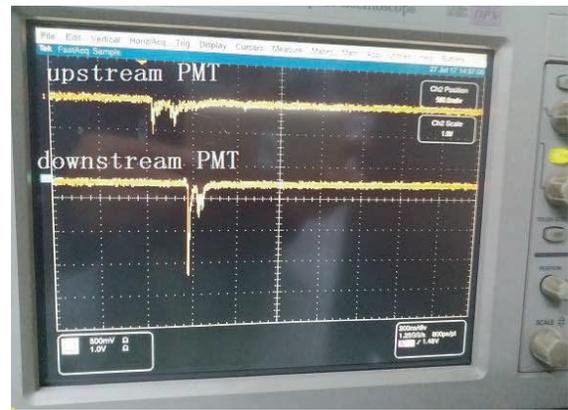
Figure 4: Typical curves of the Cerenkov light in BEPC II linac.
