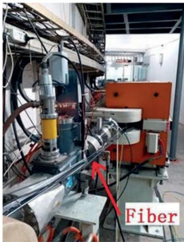
Figure 2: Black cables mounted on the side of the vacuum chamber are the optical fibers for the loss monitor.
