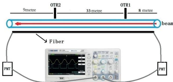
Figure 3: Scheme of the CBLM installed at BEPC II linac.
