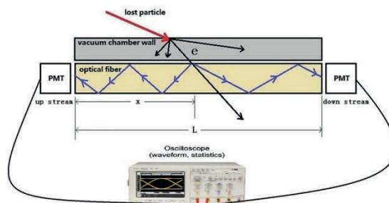
Figure 1: Scheme of beam loss monitor.
