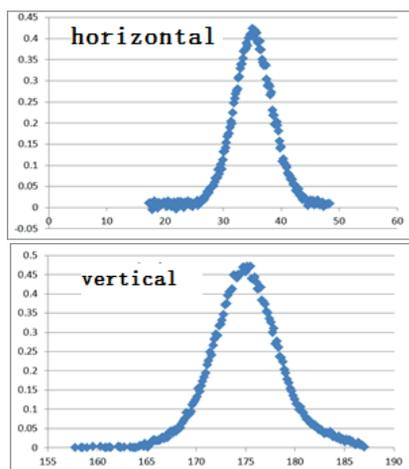
Figure 8: Beam profile measured with WS and CBLM.
