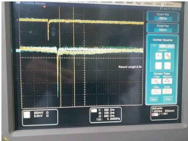
Figure 7: Beam loss generated by wire Scanner.
