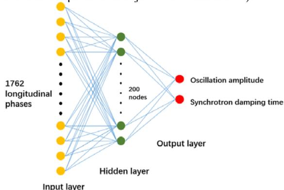
Figure 4: Schematic of the Neural network.
