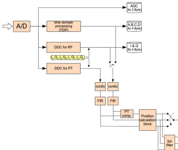
Figure 1: Processing scheme in the BPM electronics.
