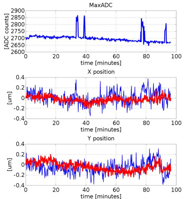
Figure 5: Transition from standard to hybrid fill pattern. Red line shows the compensated positions.
