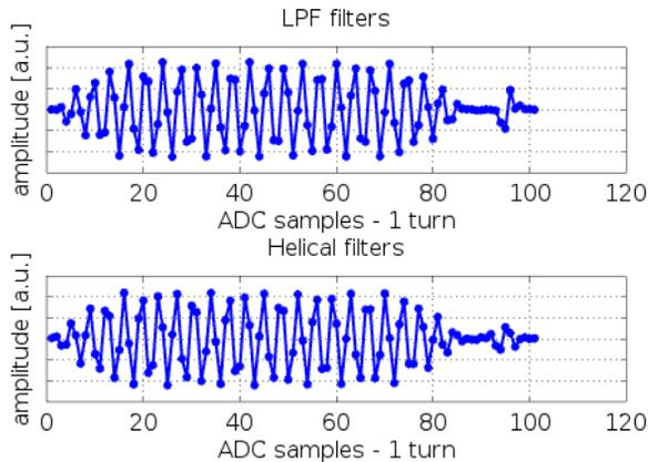
Figure 3: Comparison between the LC and helical filters.
