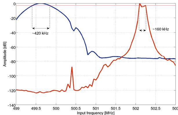
Figure 2: Digital DDC filters in the BPM electronics.
