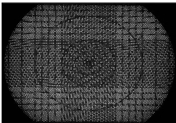
Figure 3: Acquired image with a 9 mm focal length lens (input), 10 m Fujikura FIGR-10 image fiber bundle, 25 mm focal length lens (output) and CMOS camera.
