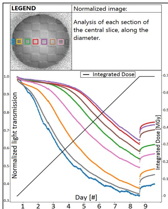
Figure 7: Transmission loss across the fibre bundle as a function of the total integrated dose.
