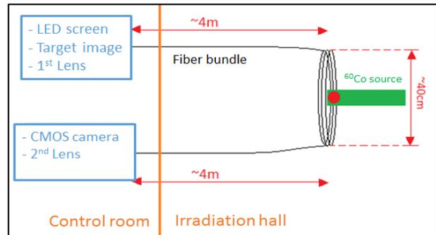
Figure 4: Sketch of the irradiation test set up.
