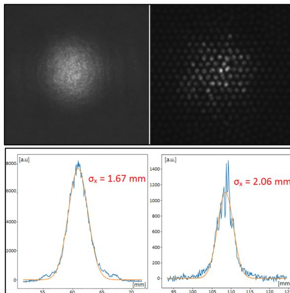
Figure 8: Laser spot image (top) and projection (bottom) without (left) and with imaging fibre bundle (right). The quoted sigma value corresponds to the width of the fitted Gaussian function.
