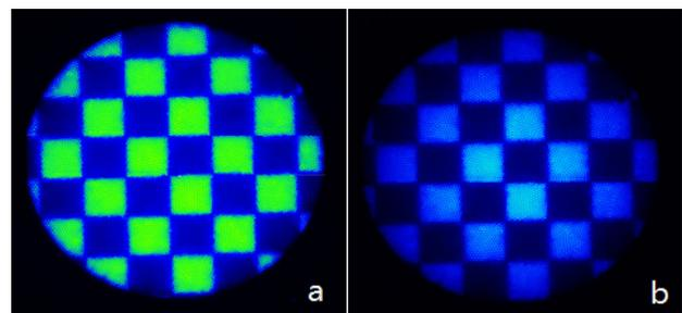
Figure 6: Test pattern image before irradiation (a) and after irradiation (b).
