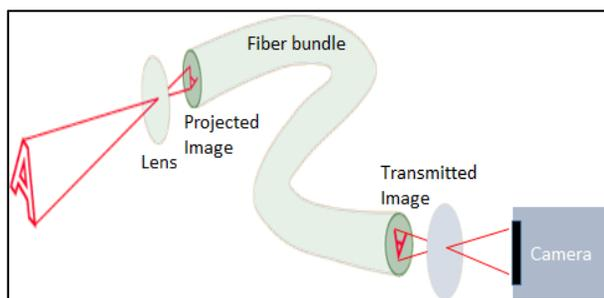
Figure 1: Sketch of the setup of the beam imaging system.
