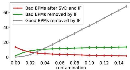
Figure 3: Adjustment of contamination factor of IF algorithm and its effect on the trade-off between cleaning of bad BPMs and removal of good ones.
