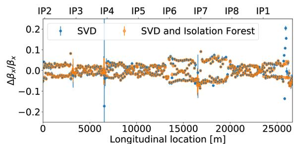
Figure 1: The comparison between beta-beating computed before and after IF cleaning demonstrates that IF anomaly detection significantly reduces the number of unphysical spikes and reduces the size of errorbars. The optics is computed for Beam 2 in horizontal plane with  $\beta^*=50$  cm.
