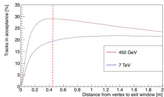
Figure 4: Percentage of tracks in the acceptance of the gas tank exit window with respect to beam gas collision distance from exit window. The dotted line corresponds to the optimum gas jet location.
