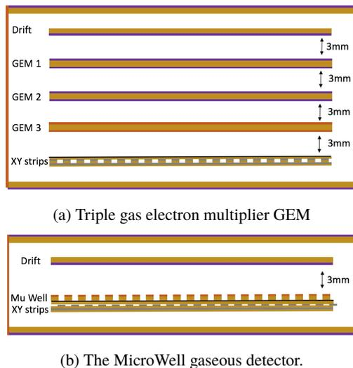
Figure 5: Sketch of the two MPGD detector candidates.
