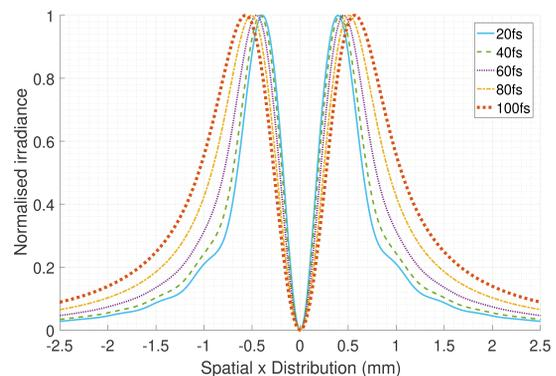
Figure 3: Comparison of the normalised simulated image distribution for different bunch lengths using beam parameters found in the MAX IV SPF.
