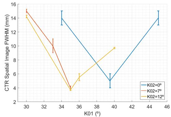
Figure 5: The effect of bunch compression on the FWHM of the CTR images.
