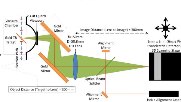
Figure 1: The single TPX lens imaging system installed in the SP02 beamline in the MAX IV SPF.
