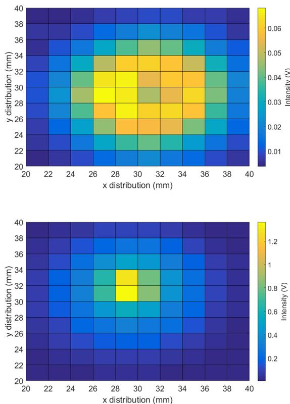
Figure 4: Example CTR images: (above) under-compressed (below) maximum compression.
