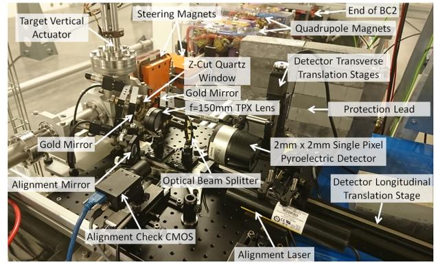
Figure 2: CTR imaging system installed on the SPF beamline at MAX IV.
