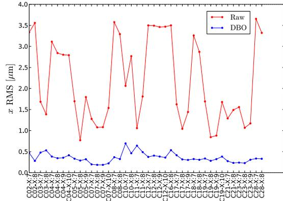
Figure 2: RMS of horizontal FA raw orbit and DBO at ID BPMs with FOFB off.
