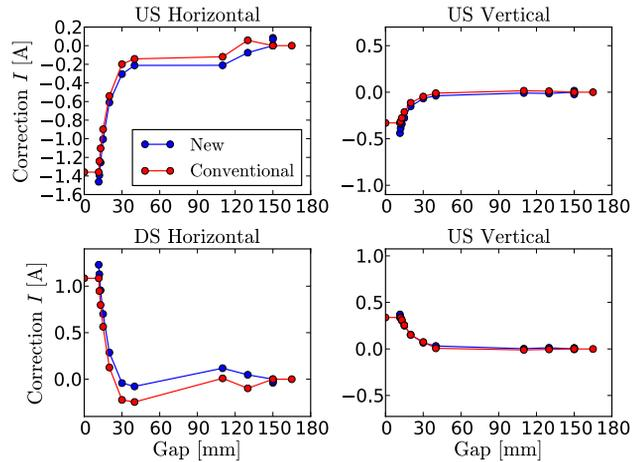
Figure 7: Orbit FF table comparison for C07 ID between the conventional and new method.
