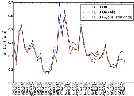
Figure 3: Comparison between FOFB off, on with and without fast correctors in BRs for RMS of horizontal FA raw orbit and DBO at ID BPMs.
