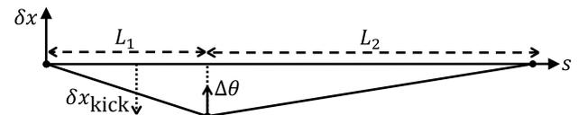
Figure 4: Relationship between a transverse kick change within BR and its effect on RSDBO.
