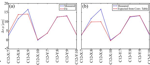
Figure 5: RSDBO for C12 ID at 6.2 mm gap. (a) Measured vs. best fit from the response matrix. (b) Measured vs. expected RSDBO from the conventional FF table.
