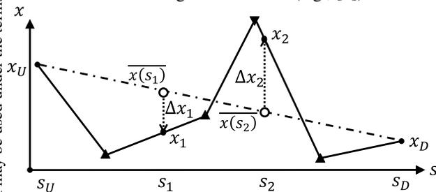
Figure 1: Schematic for dynamic orbit definitions in a region bounded by two BPMs. Triangles indicate kicks, while circles represent BPMs.
