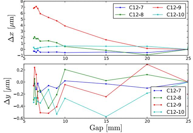
Figure 6: Estimated ID BPM physical motion with C12 ID gap motion.
