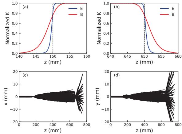
Figure 3: (a,b) Fringe field shape of quadrupoles. Electric and magnetic quadrupoles have the same length of 500 mm, The black dash lines show the edges (also Hard-Edge field). (c,d) The corresponding electron beam trajectories on the  $yz$  and  $xz$  plane.
