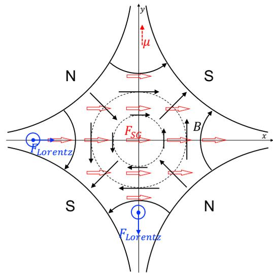
Figure 1: Field and force vectors of electrons in a magnetic quadrupole. The magnetic field vectors are indicated by black solid arrows. The Lorentz force vectors are indicated by blue solid arrows. The Stern-Gerlach force vectors, for beam polarized along the  $y$  axis, are indicated by red hollow arrows.
