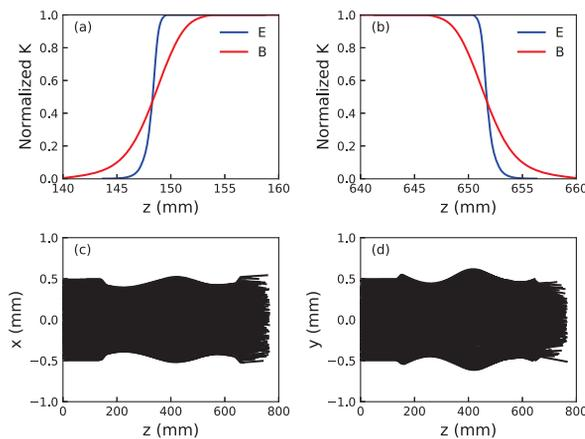
Figure 4: (a,b) Fringe field shape of quadrupoles. The magnetic quadrupole has the length of 500 mm, and the length of electric quadrupole is 502.6 mm. (c,d) The corresponding electron beam trajectories on the yz and xz plane.
