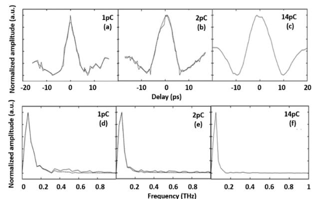
Figure 3: In the case with a laser size of 707  $\mu\text{m}$  on the cathode, the measured field autocorrelation of THz radiation for the charge 1pC (a), 2pC (b), 14pC (c), and their corresponding Fourier spectra of 1pC (d), 2pC (e), 14pC (f).
