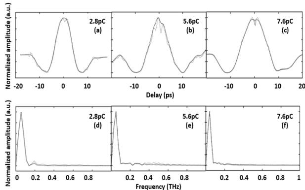
Figure 4: In the case with a laser size of 289  $\mu\text{m}$ , the measured field autocorrelation of THz radiation for the charge 2.8pC (a), 5.6pC (b), 7.6pC (c), and their corresponding Fourier spectra of 2.8pC (d), 5.6pC (e), 7.6pC (f).
