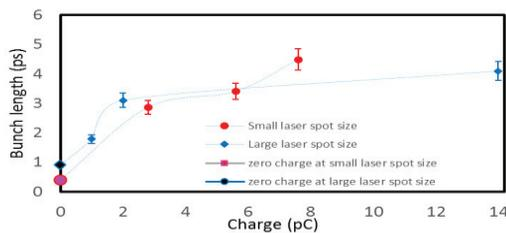
Figure 5: The bunch lengths of electron beams at two different laser sizes on the cathode 707 $\mu\text{m}$  (blue  $\diamond$ ) and 289 $\mu\text{m}$  (red  $\bullet$ ).
