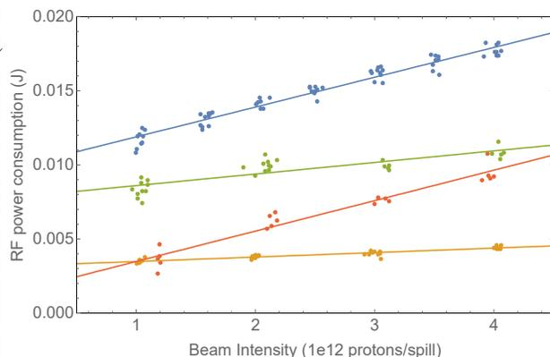
Figure 6: Estimated RF power consumption in the RF test detector. Blue is taken with atmospheric  $N_2$  gas ( $V_0 = 120 V$ ), orange is taken with 2-atm  $N_2$  gas ( $V_0 = 60 V$ ), green is tanek with 2-atm dry air ( $V_0 = 120 V$ ), and red is taken with 1-atm He gas ( $V_0 = 120 V$ ).
