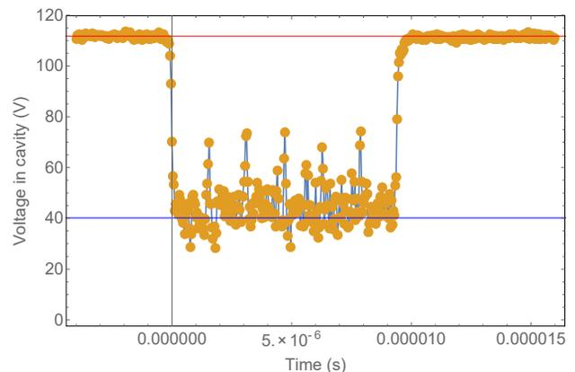
Figure 4: 1-atm N<sub>2</sub> gas-filled RF signal of a six-batches of the 120 GeV/c MI proton beam.
