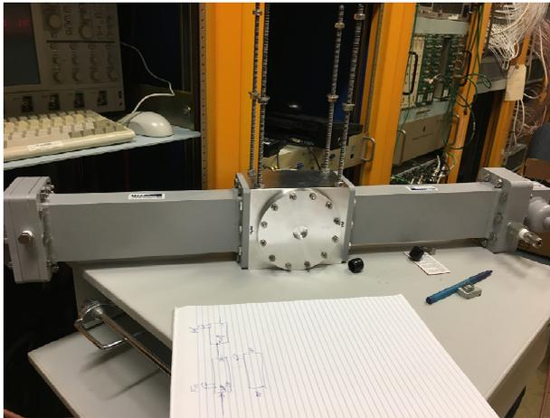
Figure 1: 2.4 GHz RF beam test detector.
