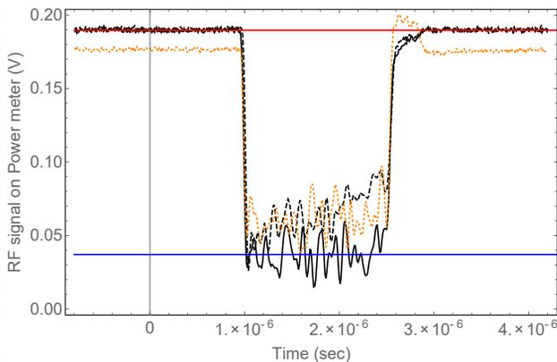
Figure 5: Four typical RF signals in the RF beam test detector with beam.
