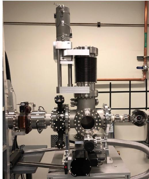
Figure 4: Assembled BID chamber. Visible from left to right: in-flange ACCT, bellows with X-Y steerer, 4-way X-Y BPM, blackened through ports on imaging octagon, 6-way cross housing full power beam dump and turbomolecular pumping, temporary beam dump with ceramic stand-offs for Faraday cup measurement of current including a cooling fan.
