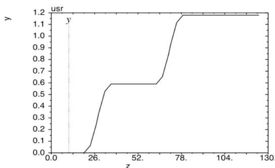
Figure 3: Vertical dogleg in the spin rotator transports the electron beam by 1.2 m in the vertical direction.
