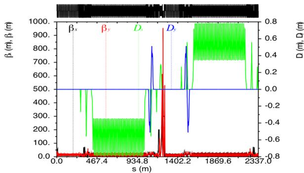
Figure 5: Complete electron collider ring optics.
