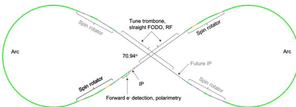
Figure 6: Electron collider ring top-view layout.
