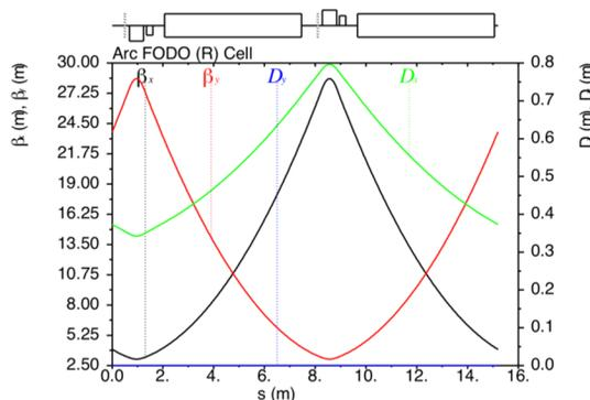
Figure 1: Electron collider ring arc FODO optics.
