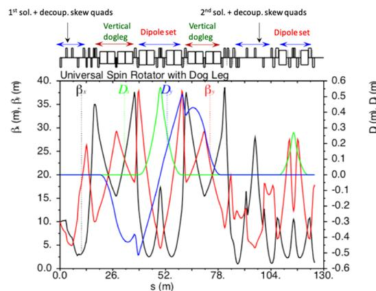
Figure 2: Spin rotator optics in the electron collider ring.
