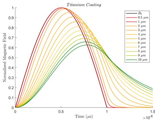
Figure 2: Field Distortion with Titanium Conductive Coating Thickness.
